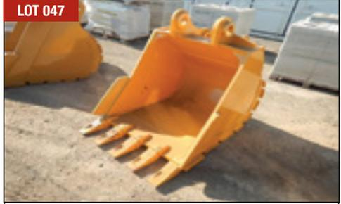
Unused 975mm Digging Bucket to suit Komatsu PC200 / Kobelco SK200
